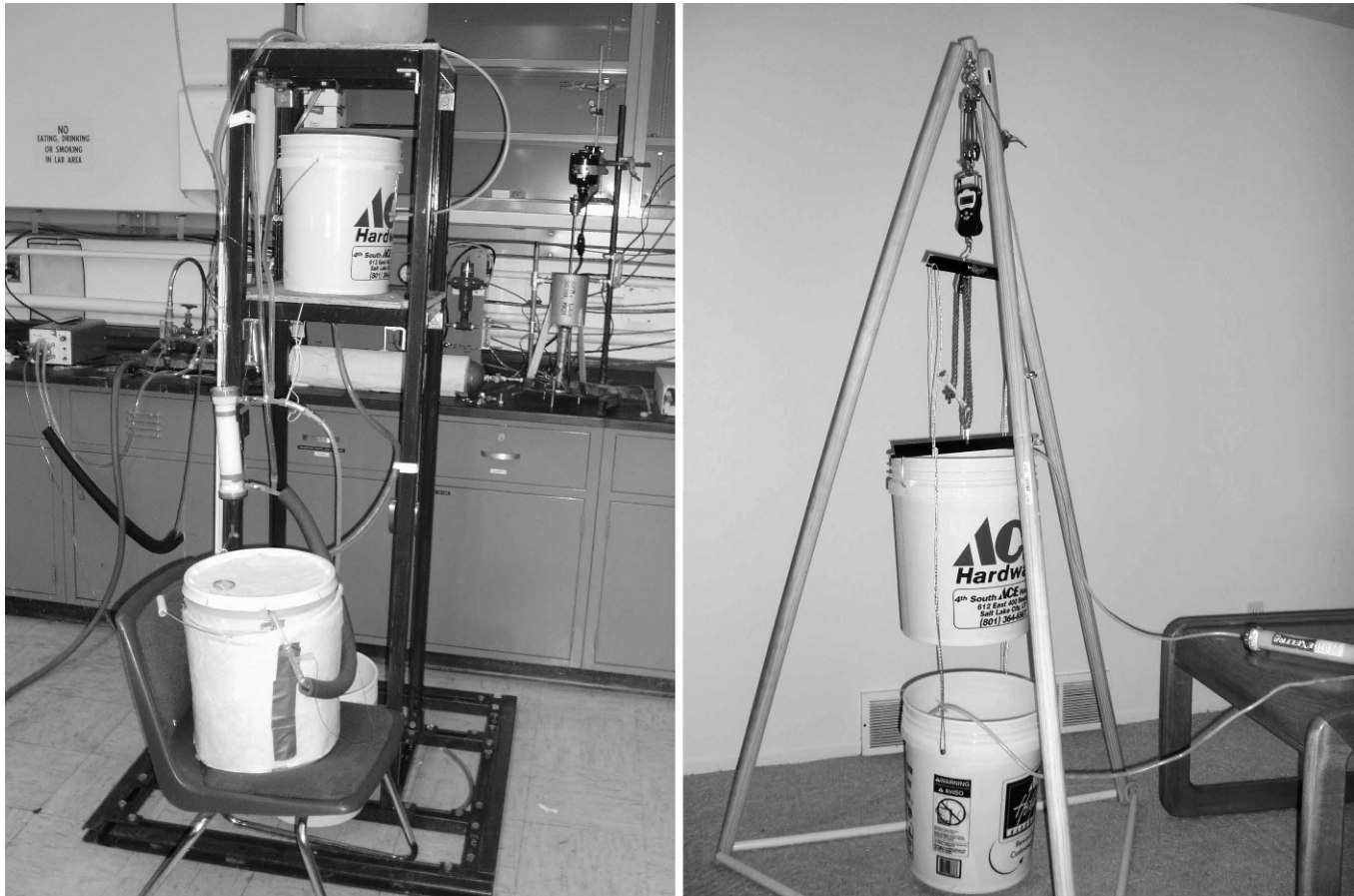
Fig 1. Prototype passive flow dialysate delivery systems. The system on the left was developed by senior students in the Department of Mechanical Engineering, University of Utah (courtesy J.J. Magda, PhD). The system on the right incorporates a mechanism for weighing the combined fresh and spent dialysate and thus monitoring ultrafiltration. In each case, dialysate flow is provided by gravity
